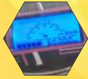
DIGITAL SPEEDO METER (BATTERY STATUS, INDICATOR, BATTERY VOLT DISPLAY, SPEED)
